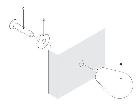
\*Drill a bolt through hole \$\Phi 4mm\$
