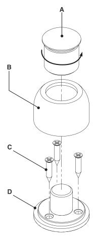
\*Drill pilot holes \$\Phi\_2\$ - 2.5mm
