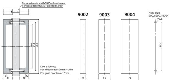
Rubber sheet and screw guide are added for the glass door.
