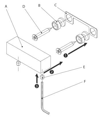
\*Drill pilot holes \$\Phi\_2 - 2.5mm\$
