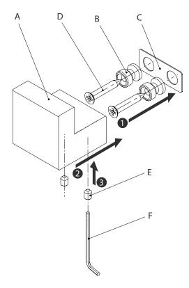
\*Drill pilot holes \$\Phi\_2 - 2.5mm\$
