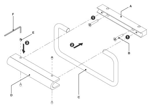
\*Drill pilot holes \$\Phi2 - 2.5mm
